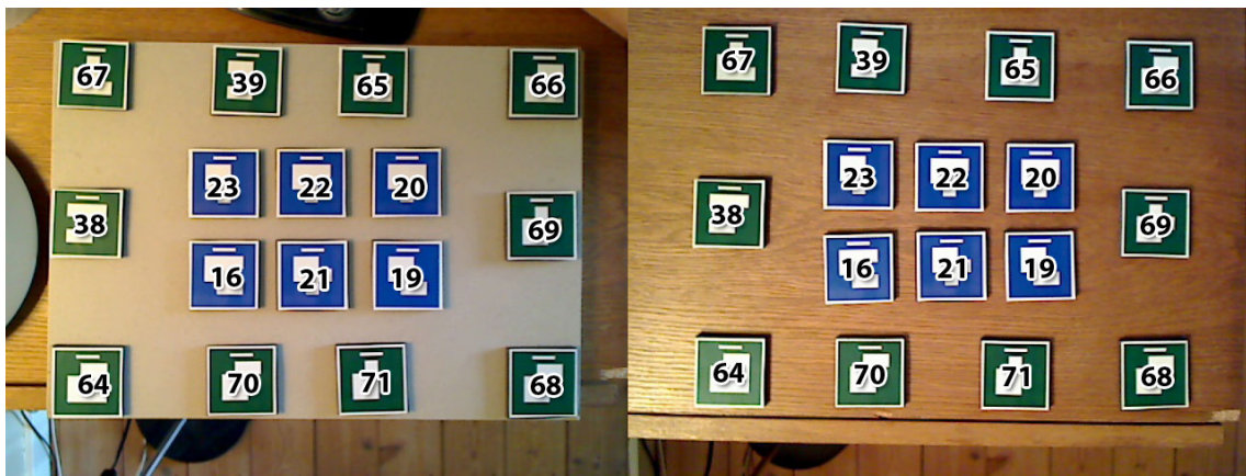
Figure 22: Tag placement on two different surfaces. The left image shows tag placement on the cardboard piece used during the game tests. The right image shows a similar tag placement, but on a table top surface. In both images the decimal value of each tag ID has been imposed to easily correlate its position and subsequent measurements in the following figures.
